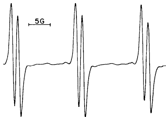
Fig. 1. ESR spectrum for the hydroxyl adduct of 4-MePyBN. Hydroxyl radicals were generated by the Fenton reaction.
